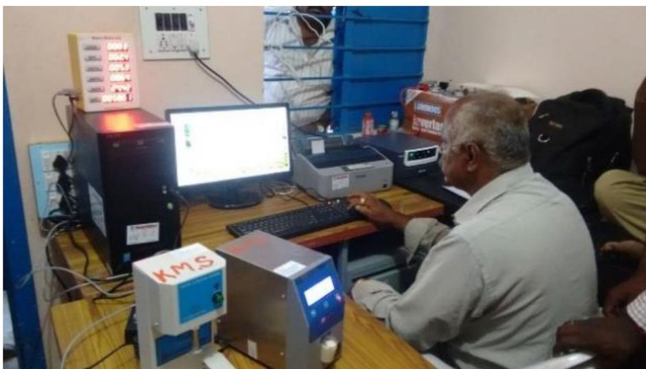
*Figure 2: Personal Computer based milk procurement system*
